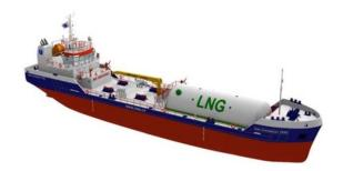
INEC1850CB is multipurpose bunkering vessel suitable of bunkering different oil products (MDO, HFO) as well LNG.
